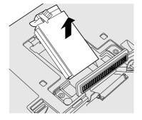
7. Open the sheet cover (G) and remove the built-in bridge battery (H). And confirm the recycle mark of the built-in battery.
